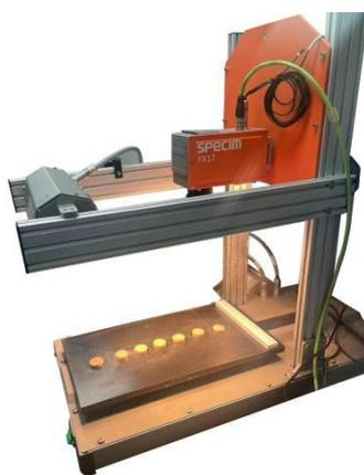
Fig. 2. Data acquisition process of near-infrared spectrometer
