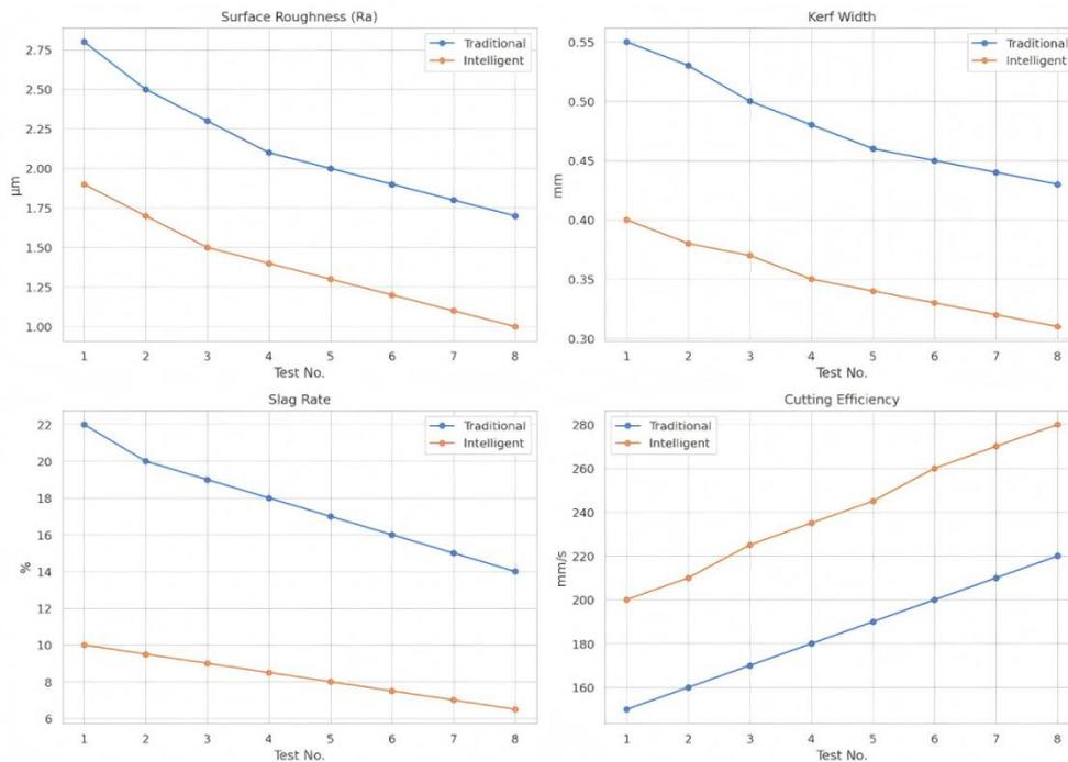
**Fig. 7.** Comparison of cutting efficiency
