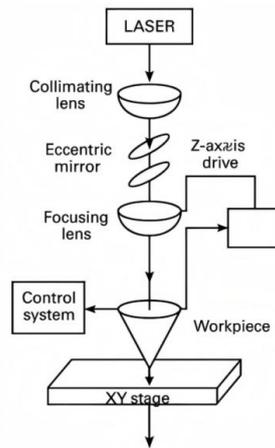
Fig. 6. Schematic diagram of the experimental platform
