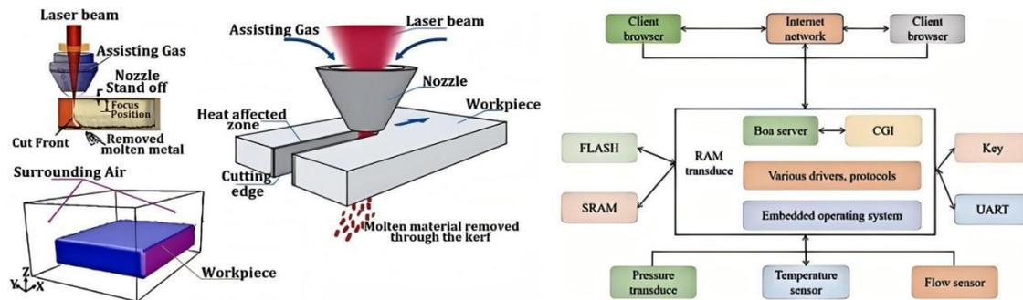
Fig. 1. Schematic diagram of the laser cutting process Fig. 2. Overall architecture of the intelligent control system
