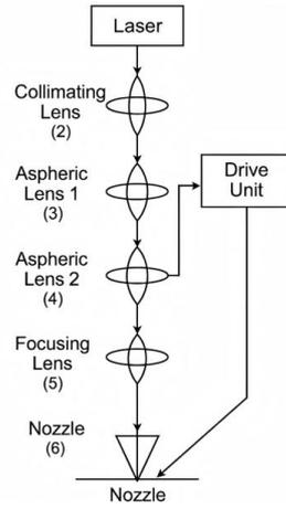
Fig. 3. The structure of the system and the laser propagation path
